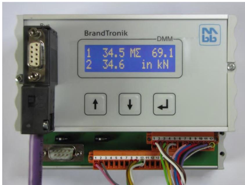
Processor based, modular structured, hybrid multichannel measuring system for transducers in strain gauge techniques.
